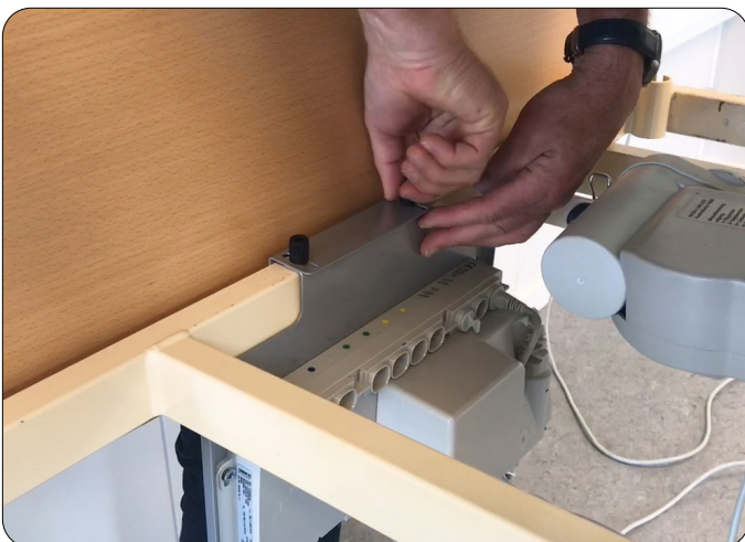
The hand control is connected to the control unit
