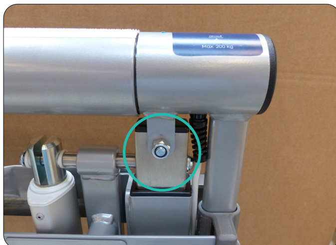
Dismount the bar from the actuator fitting
