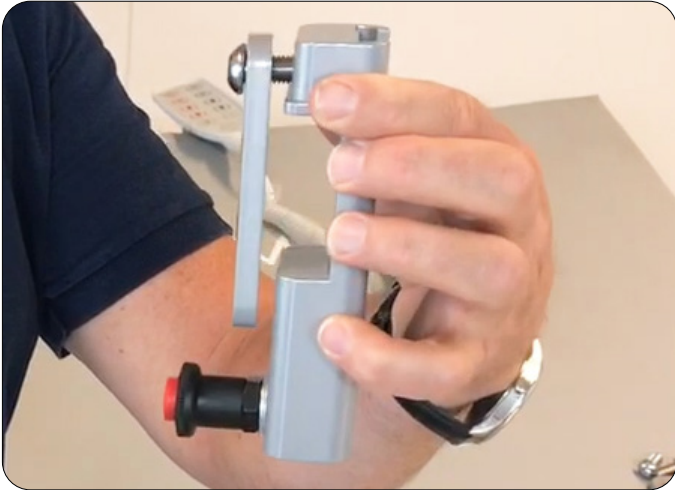
Screw the mounting plate onto the mounting bracket with the top bolt
