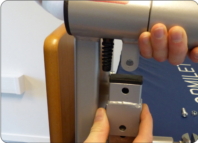
Lift up and place the height extensions
