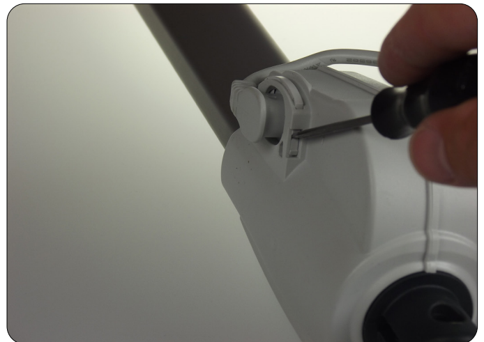
Release the locking device
