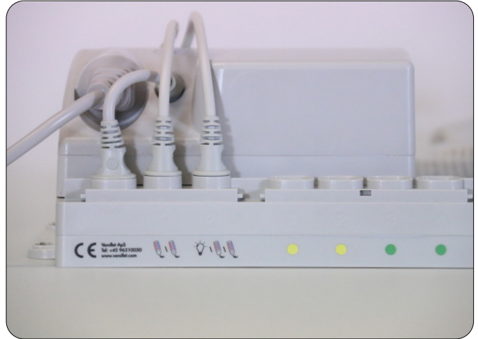
The hand control is connected to the control unit
