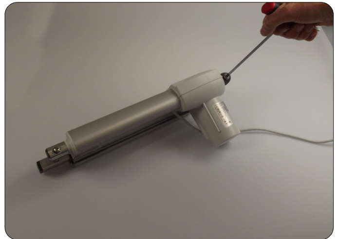
Remove the Allen screws and free the actuator
