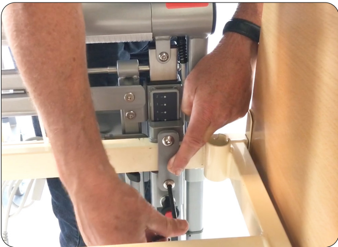
Fasten the mounting brackets by tightening both bolts
