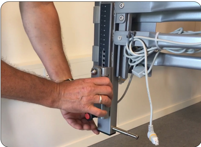
Mount the bracket on the VENDLET from the bottom up
