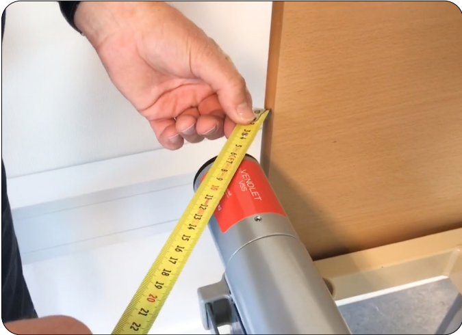
Adjust the position of the VENDLET system on the bed frame so that there is a distance of 6 cm between the head- and footboard and the VENDLET system
